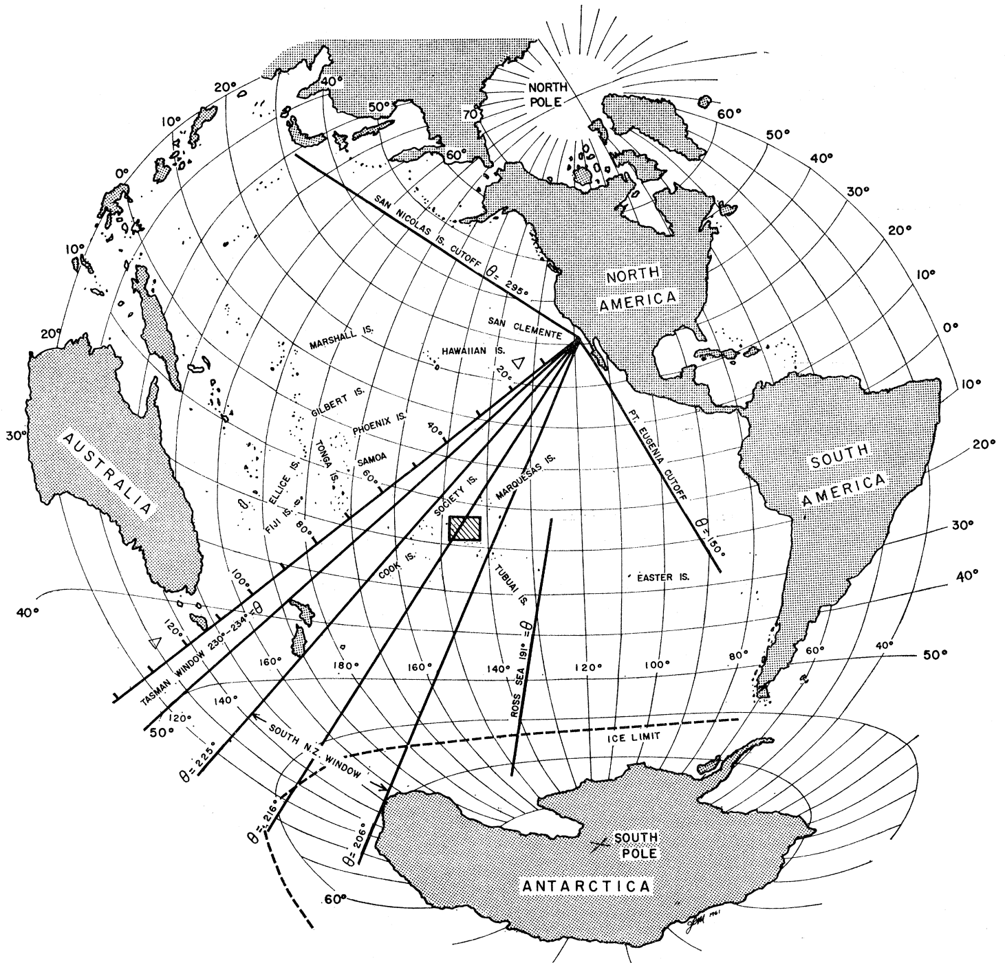
FIGURE 49. Azimuthal equidistant projection centred on San Diego, California. Some great-circle routes ( \theta = \text{constant} ) and equal distances along these ( \Delta = \text{constant} ) are indicated. The Tasman Sea and the region south of New Zealand provide two windows into the Indian Ocean, and these are partially obstructed by the Tongan and Taumotu island groups, respectively. The hatched area is shown on figure 50 on an enlarged scale. The South New Zealand window is further limited by the Antarctic pack ice.
